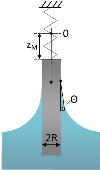
Fig. 3: Schematic side view of the platinum rod at the tip of the microprobe immersed in a test liquid
