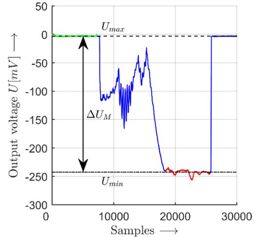
Fig. 5: Blue curve shows measured values of the output voltage  $U$  during one measurement for DI water; green/red dots show the used values for the calculation of  $U_{\max}/U_{\min}$  due averaging
