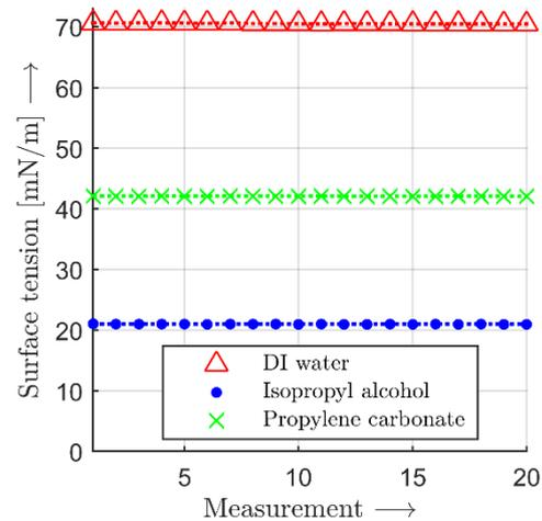
Fig. 6: Measurement results for the surface tension  $\gamma_{lv}$  of different liquids; the surface tension was determined twenty times consecutively for each liquid
