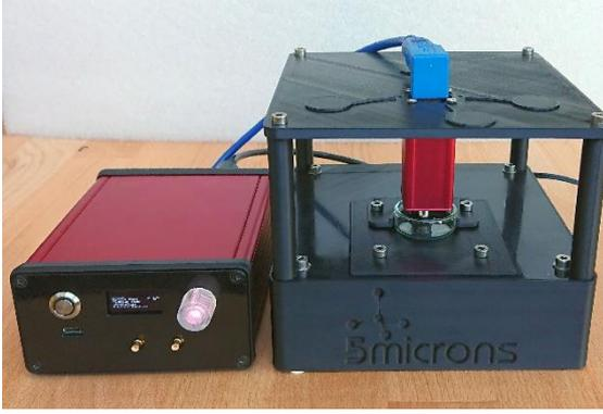
Fig. 4: Measurement system for the determination of surface tension
