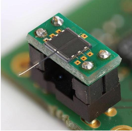
Fig. 1: Microprobe mounted on a dip socket for easy exchange; the attached platinum/iridium rod has a length of approximately  $L = 3 \text{ mm}$  and a radius of  $R = 50 \text{ }\mu\text{m}$
