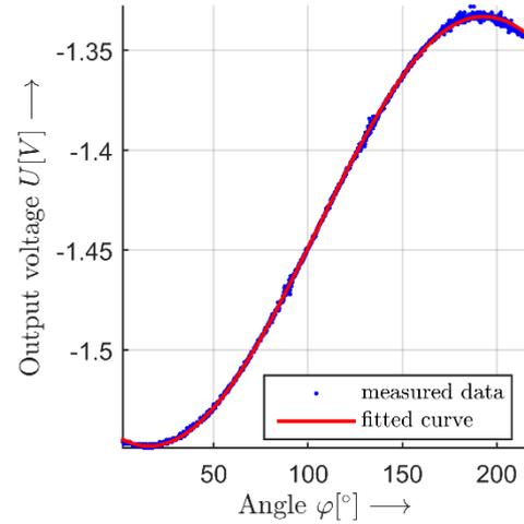
Fig. 2: Measurement data and the fitted curve  $U(\varphi) = a \cdot \cos(b \cdot \varphi + c) + d$  for the determination of the proportionality factor  $c_U$ ; the determined coefficients are:  $a = -0.1075 \text{ V}$ ,  $b = 1.0148$ ,  $c = -15.9723^\circ$ ,  $d = -1.4405 \text{ V}$
